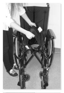
To unfold the wheelchair, move the armrests apart and push down on both sides of the seat.
